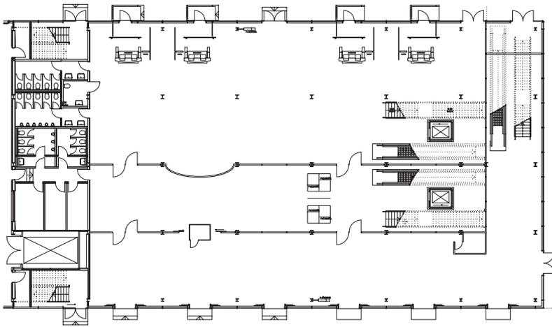
◀ At the beginning of the HIPS project over 30,000 rooms had to be assigned to the different levels. Basis were quite usable CAD data, nevertheless, they were meant for building applications. The difficulty was for automated algorithm to recognize doors and stairs from these data. As a result, the LMU scientists developed a graph-based model of the airport.
