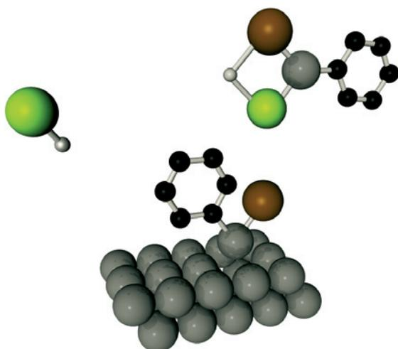
◀ The illustration shows how the lithium chloride removes the magnesium reagent stuck to the metal surface.
